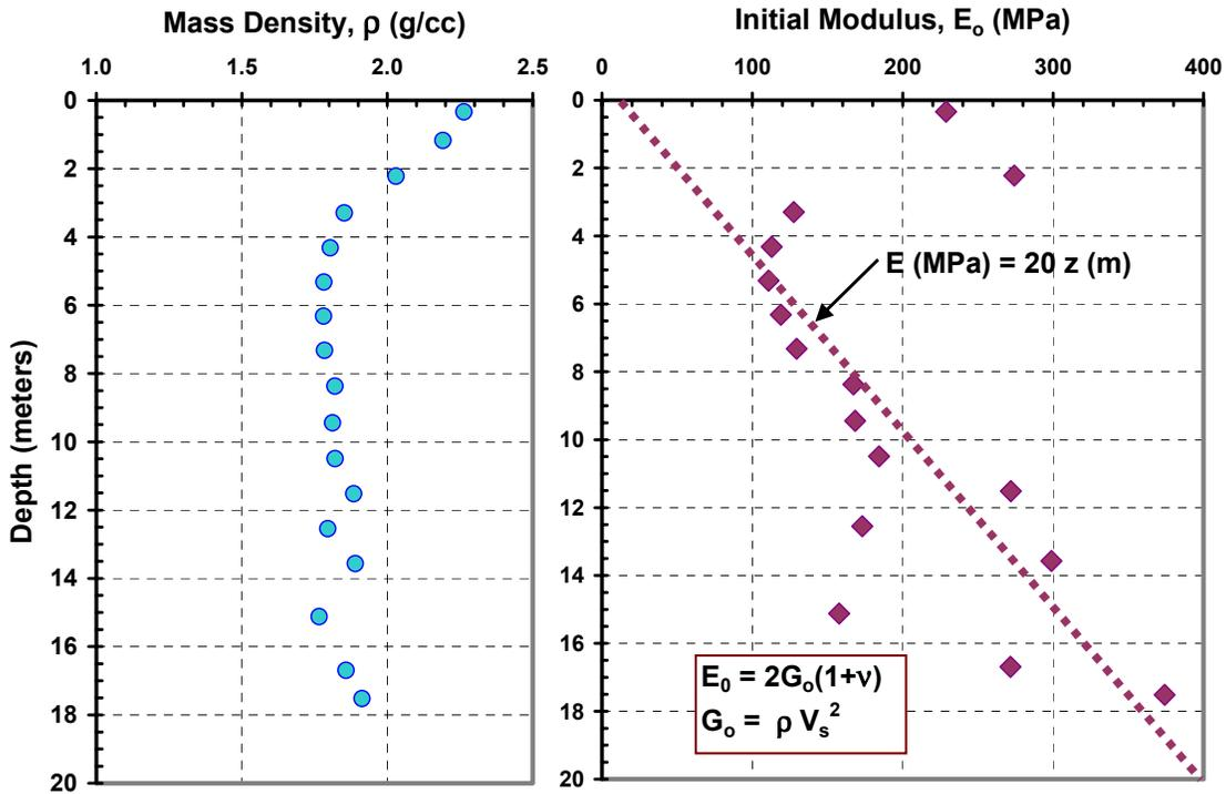
Figure 9. Derived Profiles of Density and Small-Strain Elastic Modulus at I-85.
