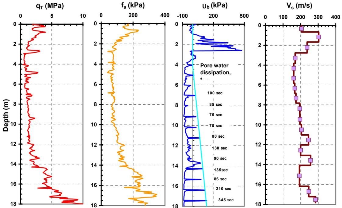
**Figure 8. Results of Seismic Piezocone Sounding at Coweta Bridge Site.**
