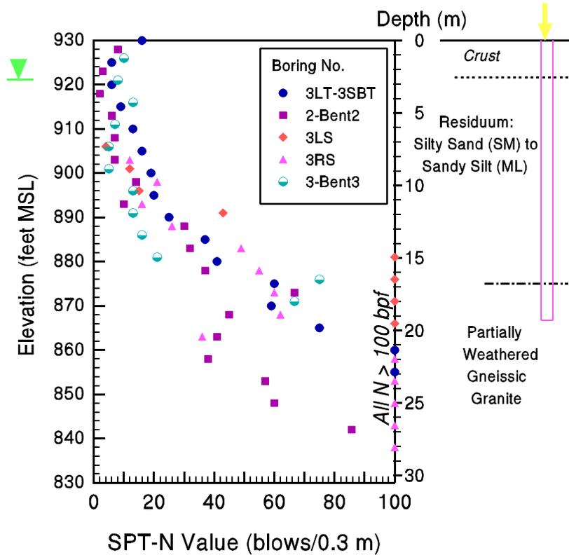
**Figure 7. SPT Summary and Drilled Shaft Profile at I-85 in Coweta County, GA.**
