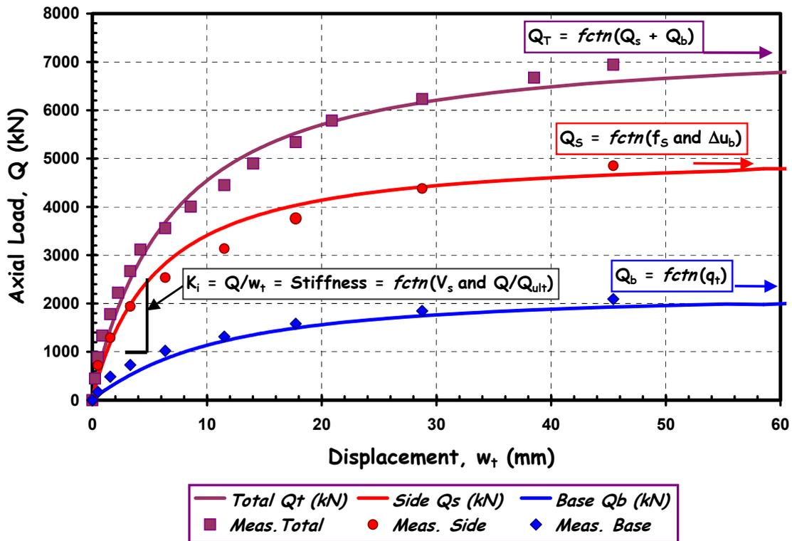
Figure 10. Measured and Predicted Load-Displacement and Load Transfer Response of Drilled Shaft at I-85 Load Test.
