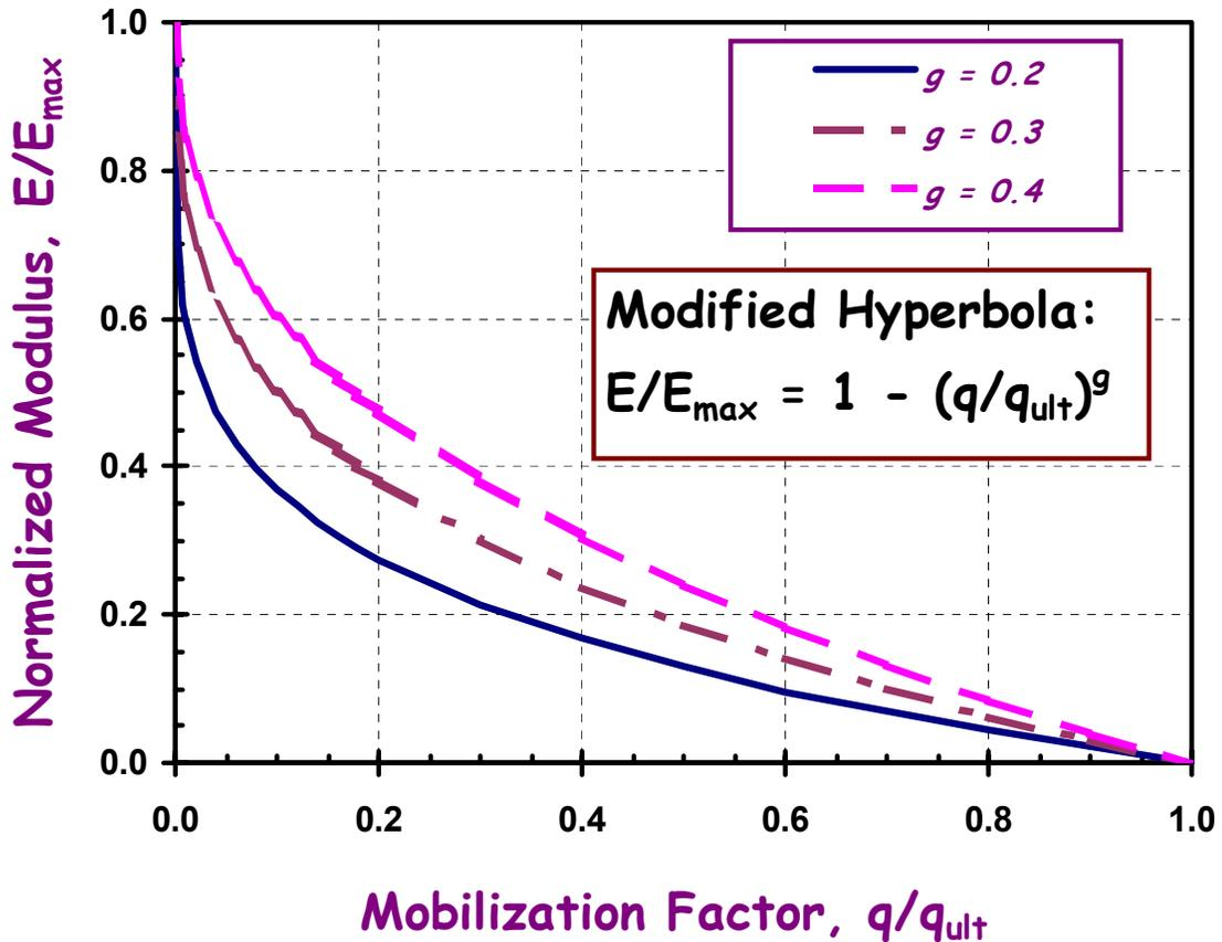
**Figure 5. Modified Hyperbolas with  $g=0.2, 0.3,$  and  $0.4$  to Illustrate Modulus Degradation Curves. Note: Mobilized stress level  $q/q_u = 1/FS$ .**
