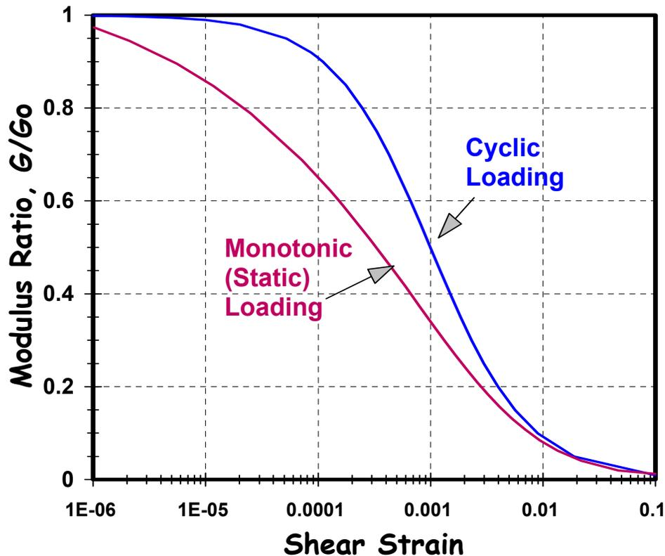
Figure 3. Modulus Degradation with Log Shear Strain for Initial Monotonic (Static) and Dynamic (Cyclic) Loading Conditions.
