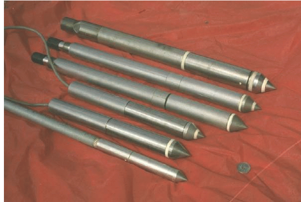
Fig. 1. Various Penetrometers (bottom to top): Miniature 4 cm 2 Electric Cone; 10 cm 2 Type 2 Piezocone (shoulder element); Type 1 (midface) piezocones; Type 2 Seismic, Hogentogler Dual Type 1 & 2 Seismic; 15 cm 2 Fugro Triple-Element Cone.
