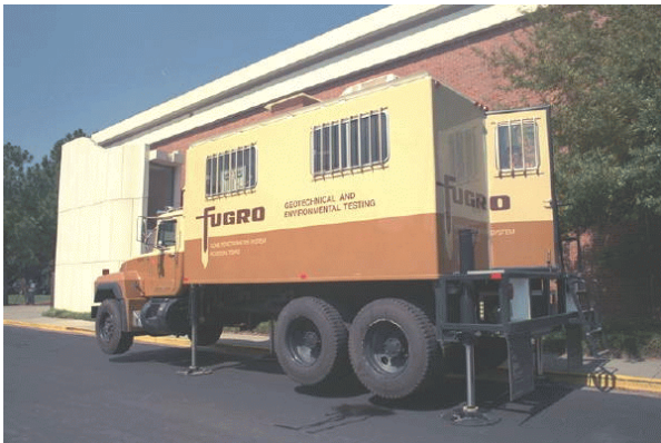
Fig. 2. Cone Truck operated by Fugro Geosciences Conducting CPTUs at Georgia Tech Civil & Environmental Engr. Building.
