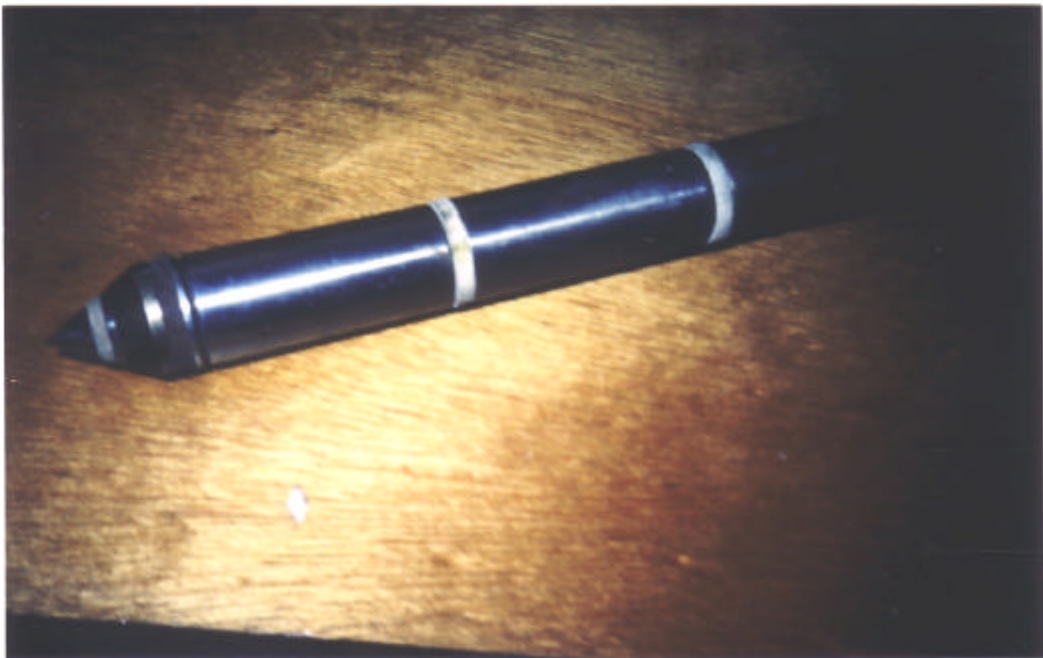
Quad-Element Piezocone (courtesy Gillian Sills, Oxford University).
