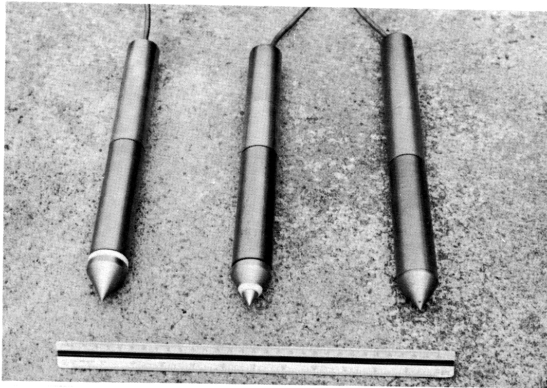
Figure A.2. L-D Type Penetrometers (from left to right) including: (a) Type 2 Piezocone, (b) Type 1 Piezocone, and (c) Standard Electric Cone.
