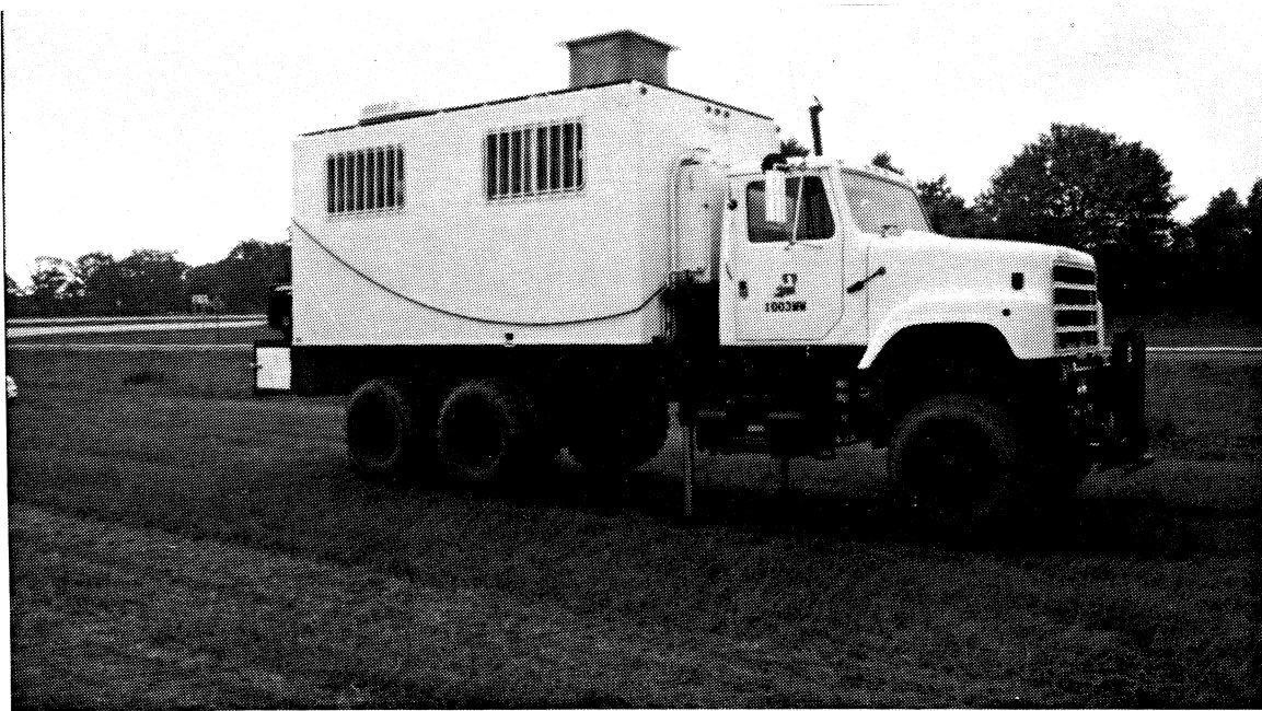
Figure 4.10. Van den Berg Type Cone Truck at Louisiana Transportation Research Center.
